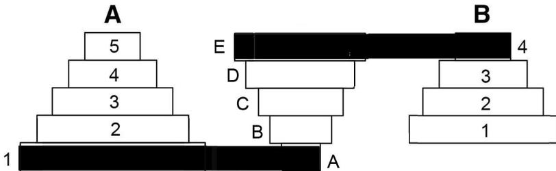
The diagram shows the belts fitted to step 1 of the spindle pulley and step 4 of the motor pulley, giving a speed of 180 rpm.
