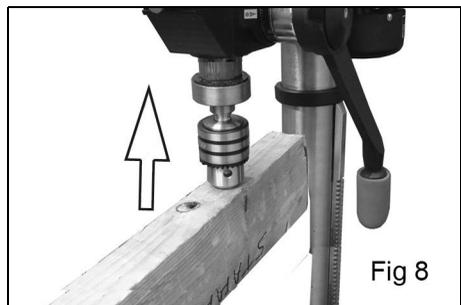
2. Tap the chuck firmly with a rubber mallet until the tapered end of the chuck engages with the drive spindle.
