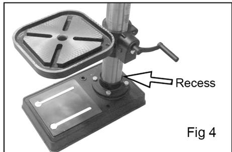
5. Fit the collar onto the column, with the recess facing downwards to hold the top of the rack in place.
