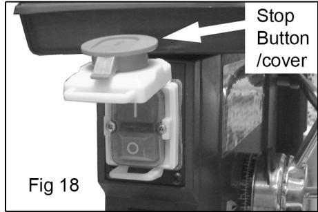
**NOTE:** As a safety feature, the ON/OFF switch is a 'No Volt Release' type. Therefore, if the power is interrupted whilst the drill press is switched ON, it will not automatically start when power is restored.
