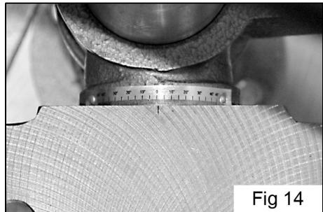
large drill bit in the chuck, place a set-square on the table, and bring it up to the drill. Adjust the table if necessary, so that it is perfectly level.
