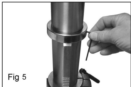
7. Ensure there is sufficient clearance to allow the complete table assembly to move around the column. If necessary, reposition the collar to achieve good movement.
