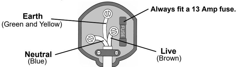
**Ensure that the outer sheath of the cable is firmly held by the clamp**
