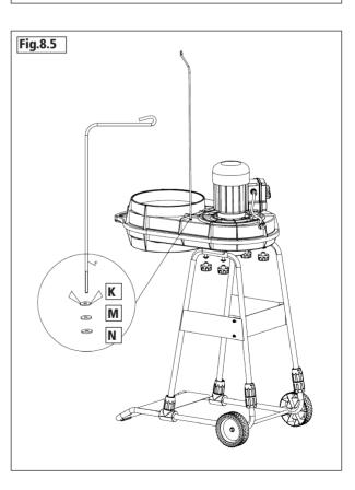
6. Thread the butterfly nut (K) onto the bag support arm. Place the spring washer (M) and washer (N) on the bag support arm and screw the bag support arm to the motor and housing, Fig 8.5. Lock the arm in position using the butterfly nut.
